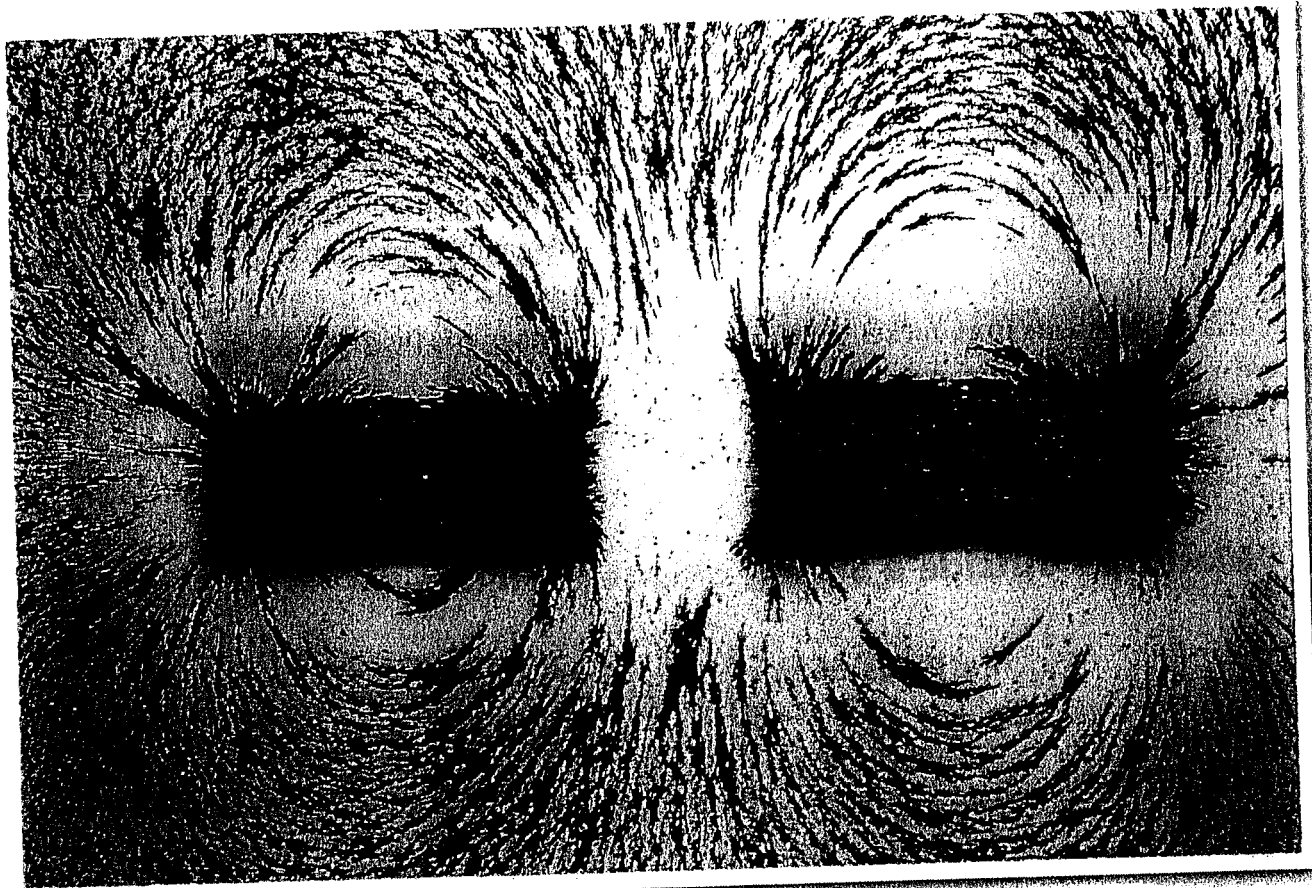
Iron filings spread around a magnet will form a pattern that shows the shape of the magnet's magnetic field.
